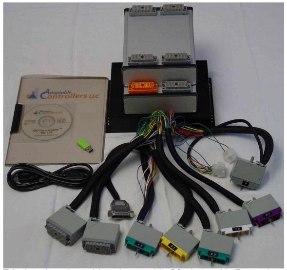
This photo shows the module enclosure and the BC adapter cable. To see other enclosures and adapter cables, click on the corresponding link below.
